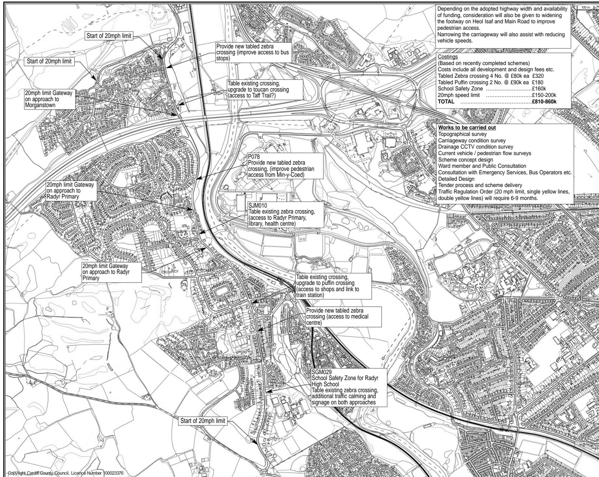
Depending on the adopted highway width and availability of funding, consideration will also be given to widening the footway on Heol Isaf and Main Road to improve pedestrian access. Narrowing the carriageway will also assist with reducing vehicle speeds.
